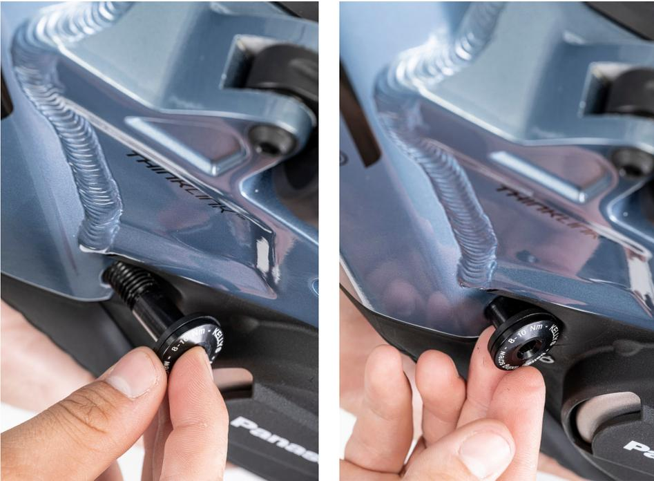
FIGURE 9: VIS INTRODUITE DANS LE CADRE
