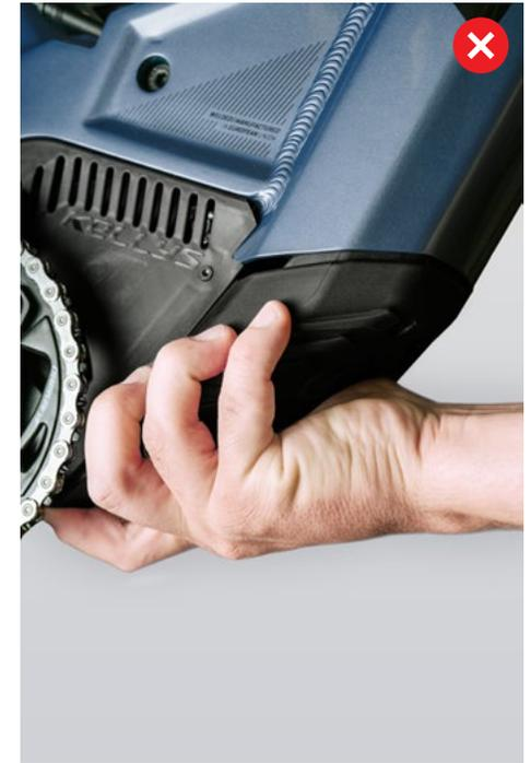
FIGURE 8: VÉRIFIER QUE LE CAPOT DU MOTEUR EST RECOUVERT PAR LE CAPOT DE LA BATTERIE SUR LE CÔTÉ DROIT (CÔTÉ ENTRAÎNEMENT)
