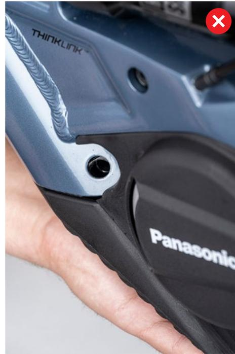
FIGURE 7: VÉRIFIER QUE LE CAPOT DU MOTEUR EST RECOUVERT PAR LE CAPOT DE LA BATTERIE SUR LE CÔTÉ GAUCHE (CÔTÉ FREINS)
